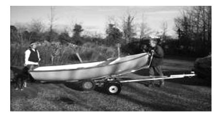
c) The boat should be tied down to the road trailer by the painter. A ratchet strap or rope should be passed over the boat between the shroud plate and the foredeck secured to the forward trailer "D" rings and tensioned. Do not over tension the ratchet straps. When using rope, pad the gunwales and make a Trucker's Hitch in the standing part to provide additional purchase.
