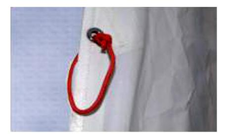
a) Attach a reefing loop to the reefing cringle in the luff of the sail and pass it over the end of the boom.
