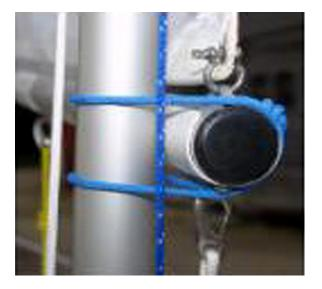
e) When not using a jib it can be advantageous to attach the downhaul to an eye approximately 200 mm from the front of the boom. This allows the boom to project forward of the mast and can improve performance.
