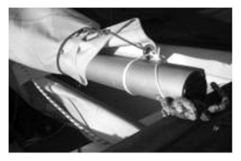
b) Pass the leech reefing line through the clew cringle and back through the leech cringle, tension it and tie off round the boom. This will hold the reef down and flatten the sale.
