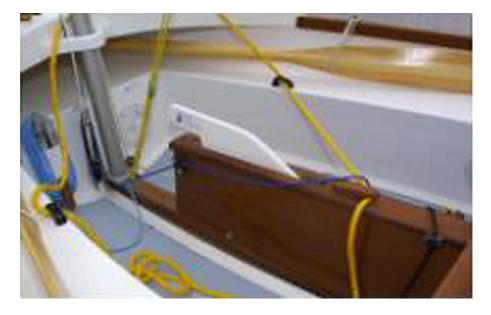
Rowlocks are stored in pockets under the thwart and the oars are released by unclipping the hooks on the shroud plates.
