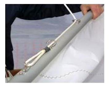
d) After hoisting, the surplus sail can be kept tidy by tying up the three reefing lines round the boom.
